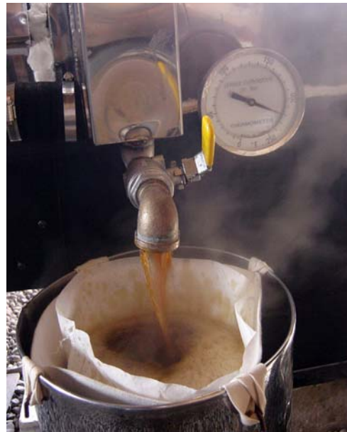
Drawing off a batch of finished syrup from CNC's modern evaporator pan in the Sugarhouse
